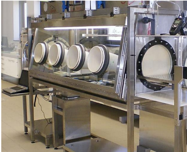
Figure 10: Negative Pressure Glove Box. Note the direction that the gloves are facing.
