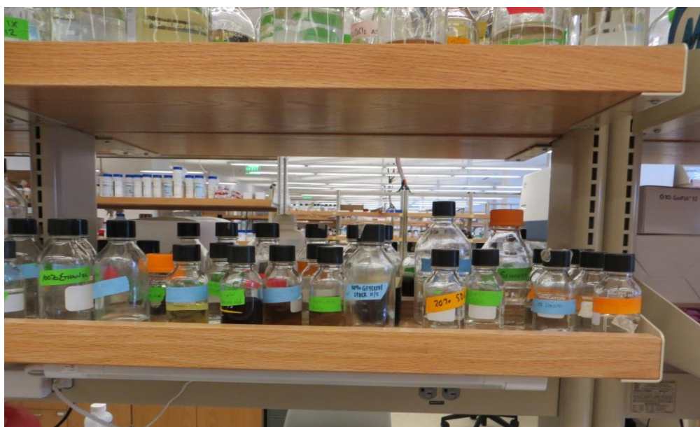
Figure 46: Chemical labeling. Even when there are large numbers of bottles, all of them must be labeled as in the picture.
