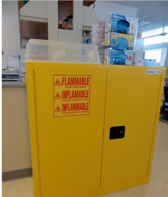
Figure 53: Flammables cabinet. Flammables cabinets should be closed unless removing a chemical. Items should not be stored on top of them.
