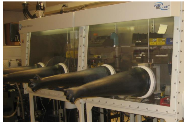
Figure 11: Positive Pressure Glove Box. Note the direction that the gloves are facing.
