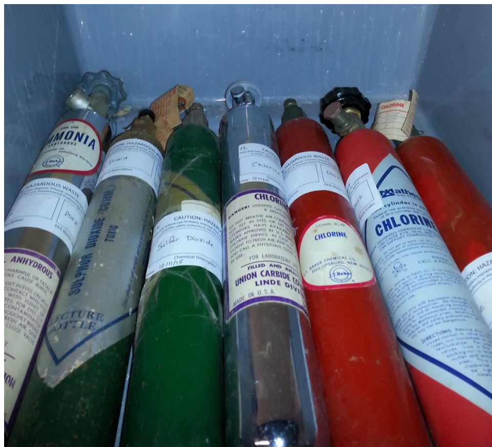
Figure 62: Lecture Bottles. Lecture bottles are small compressed gas cylinders; many of them contain highly hazardous chemicals like those pictured above. Use storage and disposal of these types of gases is both complicated and expensive. EHS should be consulted before ordering lecture bottles of hazardous gases.
