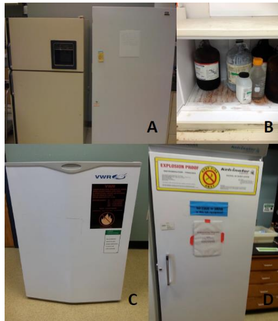
Figure 54: Laboratory Refrigerators and Freezers. A-Standard refrigerator and freezer. Any refrigerator that looks like it came from an appliance store is not approved for the storage of flammables. B-Improperly stored flammables. Flammable materials must not be stored in standard refrigerators or freezers. C and D- Flammable storage refrigerators and freezers. These are readily identified by markings on front.
