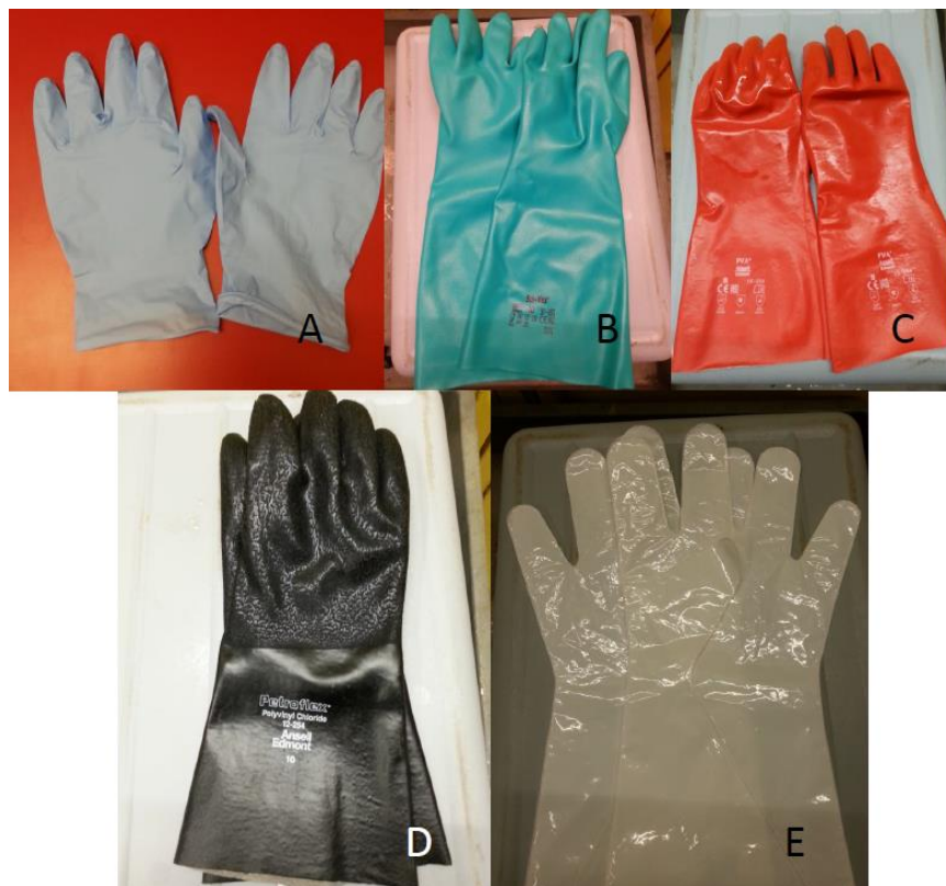
Figure 29: Gloves for chemical hazards. A-Standard nitrile gloves. These are the most common laboratory gloves and they are suitable for use with most chemicals. They are unsuitable for use with halogenated solvents, acetone, phenol or benzene. For complete compatibility discussion, see manufacturer's chemical resistance guide. B-Solvex gloves. These gloves are made of the same material as nitrile; they are just thicker and longer. This thickness reduces dexterity but increases protection. C-Polyvinyl alcohol (PVA) gloves. PVA gloves are should be used when large amounts of halogenated solvents (like chloroform) are going to be used. These gloves have limited dexterity and are expensive (~$30 per pair). D-Polyvinyl chloride (PVC) gloves. PVC gloves tend to be more susceptible to chemical breakthrough than nitrile, but there are a few chemicals for which they are more protective than nitrile (like phenol). E-Laminate film gloves. These gloves are resistant to almost every chemical; however, they have very limited dexterity. They should be used as a last resort in a laboratory setting but are good for used in chemical spill cleanup kits.
