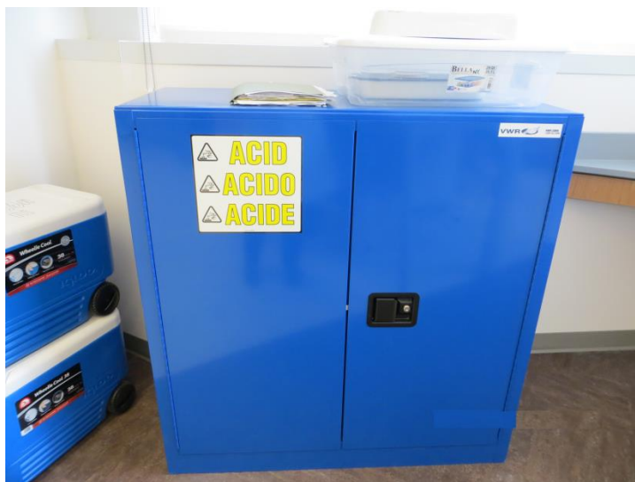
Figure 55: Corrosive Storage Cabinet. These cabinets are suitable for storage of corrosive materials like acids and bases. If acids and bases will be stored in the same cabinet, each has to be in its own secondary container to prevent the possibility of the two mixing in the event of a leak or spill.
