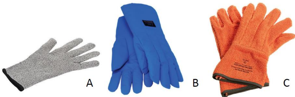
Figure 27: Gloves for physical hazards. A-Cut-resistant gloves. Cut resistant gloves should be used for tasks involving sharps such as syringes, razor blades and scalpels. These gloves are fairly flexible and do offer some dexterity. B-Cryogenic gloves. These gloves should be used with cryogenic liquids when possible. C-Autoclave gloves. While these gloves are called autoclave gloves, they may be used for handling hot items from ovens and hot plates as well.
