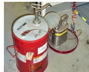
Figure 51: Appropriately Grounded and Bonded Containers.
