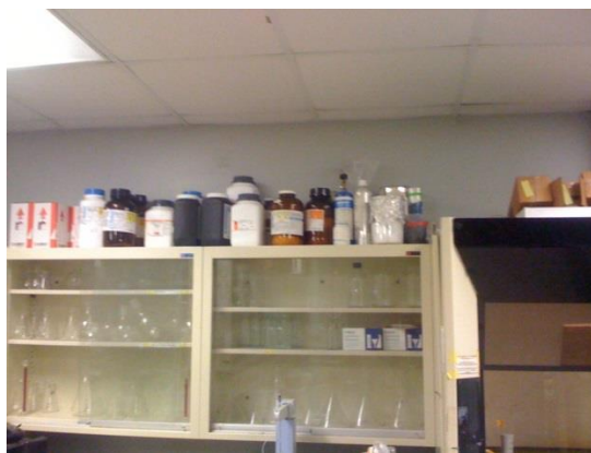
Figure 48: Improper Chemical Storage on a High Shelf. Chemicals should not be stored this high; especially chemicals in such large containers! The chemicals should be in the cabinets that in the picture have glassware stored in them.
