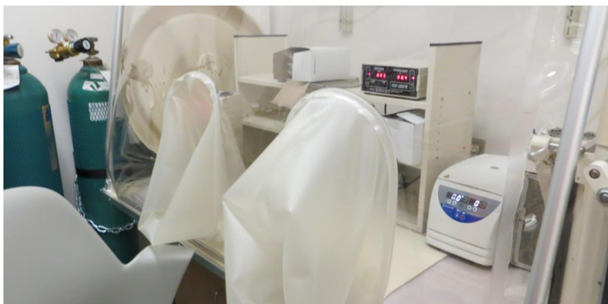
Figure 12: Glove Bag. Materials are placed in the airlock on the far right; the airlock is purged with an atmosphere free of oxygen. Once the purge is complete, materials are then taken into the main chamber. Note the percentage of hydrogen in this bag is 4% according to the gauge.
