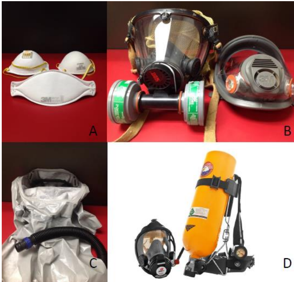
Figure 31: Examples of respirators. A-N95 dust masks. These are several different types of dust masks that are all considered respirators by OSHA. B-Full-face air purifying respirators. These respirators require cartridges that filter out different types of contaminants (dependent on the type of cartridge). They provide a higher level of protection than a simple dust mask. C-Powered air-purifying respirator (PAPR). This hood attaches to a pump that filters air to remove contaminants. Unlike the other types of respirators, it is loose fitting. D-Self-contained breathing apparatus (SCBA). This type of respirator isolates the breathing air into a tank. These types are not used in the laboratory, but are appropriate for many emergency response situations.
